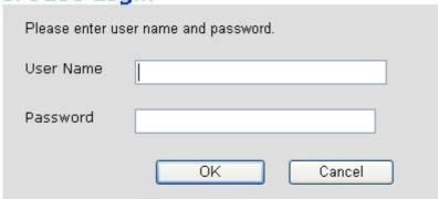
Type the new IP address of IP Power 9258 in the address field and you can enter the login web page. Input the default password 12345678, or the password set by you, click **OK**, and you can then enter the Web Control page.
